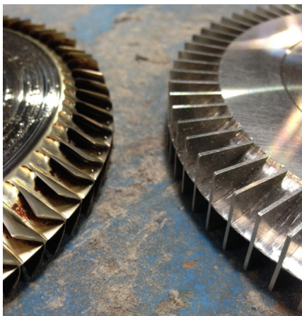
Picture 2: New impeller (right). Impeller after three months of use (left). Worn caused by residual plastic chips is clearly visible on the old impeller
