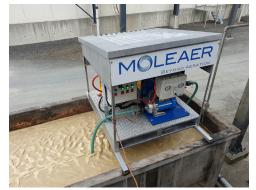
Moleaer's nanobubble generator is compact, and easy to install without retrofitting the existing system.
