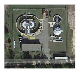
Aerial view of 3-ring oxidation ditch system at the Village of Warrens (WI) treatment plant.
